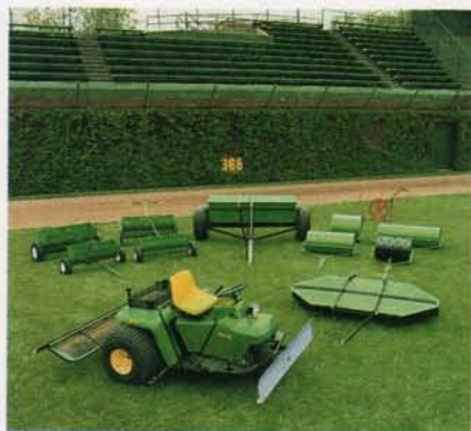
Attachments such as seeders, spreaders, brushes, blades, scarifiers and rakes help the 1200 work productively on any ball field.
