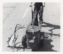
The TMS-4 self-propelled striping machine has a simple friction drive system. Powered by an eight-hp air-cooled engine and a 13.2 cfm twin-cylinder cast iron compressor, the unit can spray a single one- or two-inch wide line or two six-inch parallel lines simultaneously.
