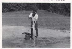
The Diamond Pump quickly removes standing water from infield puddles. Lightweight and easy to use, the pump will not clog from mud or dirt.
