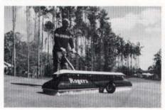
The 80-inch Greensfoil Hosefed Walking Boom has mechanical drift control, which allows spraying in windy conditions. Its advanced airfoil protects the operator and environment and ensures positive drift control.
