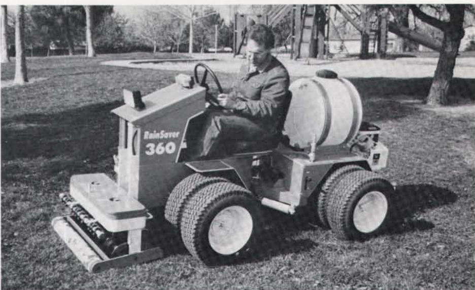
RainSaver injects a gel of starch-based polymers into the rootzone.
