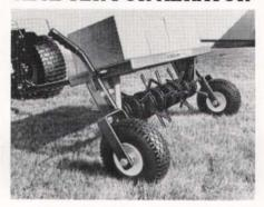
A three-point hitch adapter can be used with Feldmann's Model 2340-32 or Model 2340-48 core plug pull-behind aerators. Using a tractor's hydraulic power, it enables the aerator tines to be raised and lowered.
