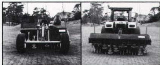
The 305.200H and 305.250 both use 16" deep tines. The 305.200H has a working width of 79" while the 305.250 is at 98".
