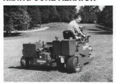
With a 52-inch swath and 60,000-squarefoot-per-hour capacity, the Ransomes Riding Core Aerator is ideal for aerating large greens and fairways. Its wide, smooth tires and three-wheel design distribute weight evenly, minimizing turf marking.
