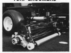
For greater strength and durability, the Jacobsen Turf Groomer has a large front roller and large, thick six-point cutting blades. Previously designed for greens conditioning, a model for fairway use has also been introduced by the company. Two blade spacings are available.
