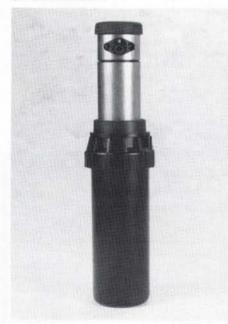
Designed for sports fields, golf courses, cemeteries, and other large turf areas, the I-40-ADS adjustable arc sprinkler can be set at any arc between 40 and 360 degrees. Arc adjusment can easily be made with the water on or off.
