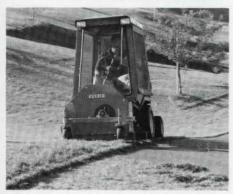
The F2400 front mower is equipped with a 24-hp, four-cycle, three-cylinder, vertical liquid-cooled diesel engine. The unit's hydrostatic transmission works together with its front differential lock and fourwheel-drive to provide traction and smooth operation on uneven or slick terrain. In addition, the hydrostatic transmission permits the operator to easily select ground speed.
