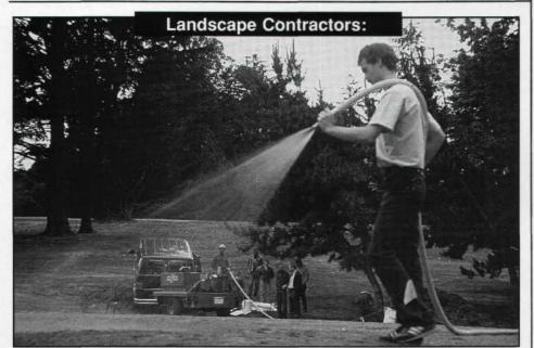
Bowie Hydro-Mulcher® delivers the heaviest slurries of seed, fertilizer and mulch without plugging.
