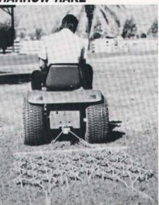
The unique four-foot Harrow Rake from Farnam Equipment Companies is designed specifically to clean up and renew choked-out lawns. Growth is stimulated by allowing better penetration of air, water and nitrogen.
