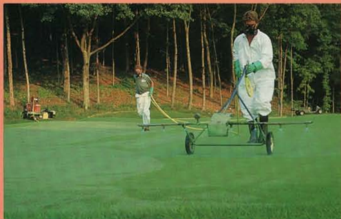
Walk-behind boom sprayer applies fungicide mix to greens.
