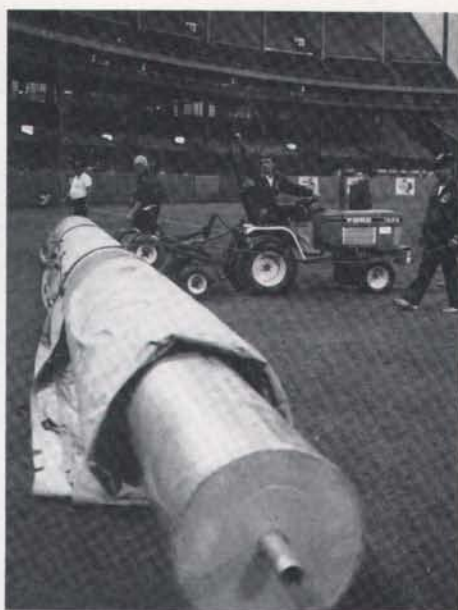
Six men can remove tarps with the help of a tarp machine developed by Frey.
