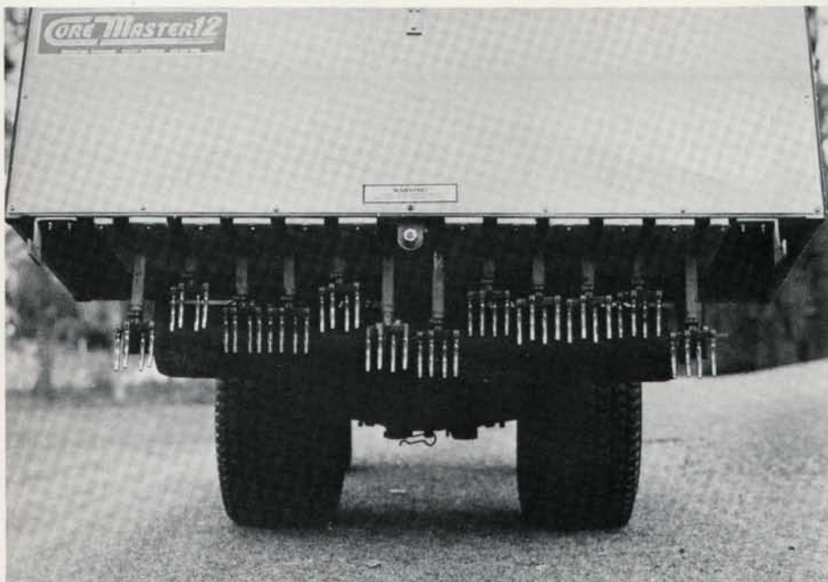
Closeup of quadratines on Green Care CoreMaster 12.
