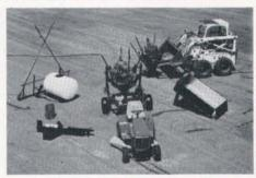
The flexibility of small tractors or loaders can be increased with the Dakota Hand transplanter frame by Mid-Dakota Corp. The unit's frame is adaptable in minutes to fit a tree spade, sprayer, hydraulic dump wagon, log splitter and post hole digger. A towable model is available for tractors with threepoint hitches and a bucket-mount model can be attached to loaders.
