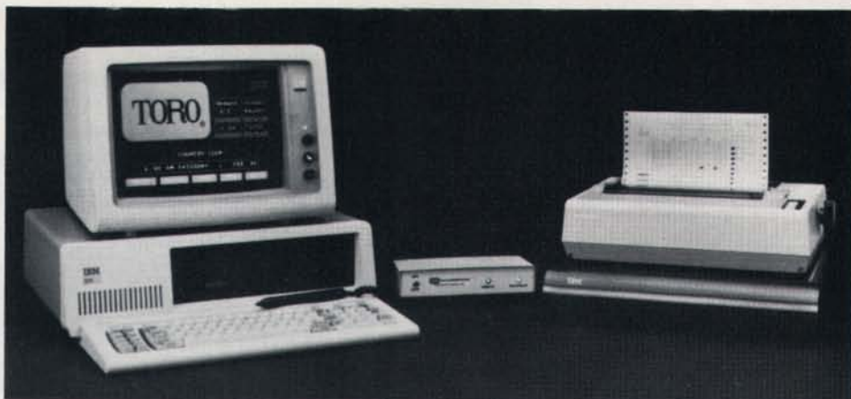
The heart of the Network 8000 is an IBM/XT personal computer. A phone modem links the computer to the satellites and a printer provides "hard copy" reports.
