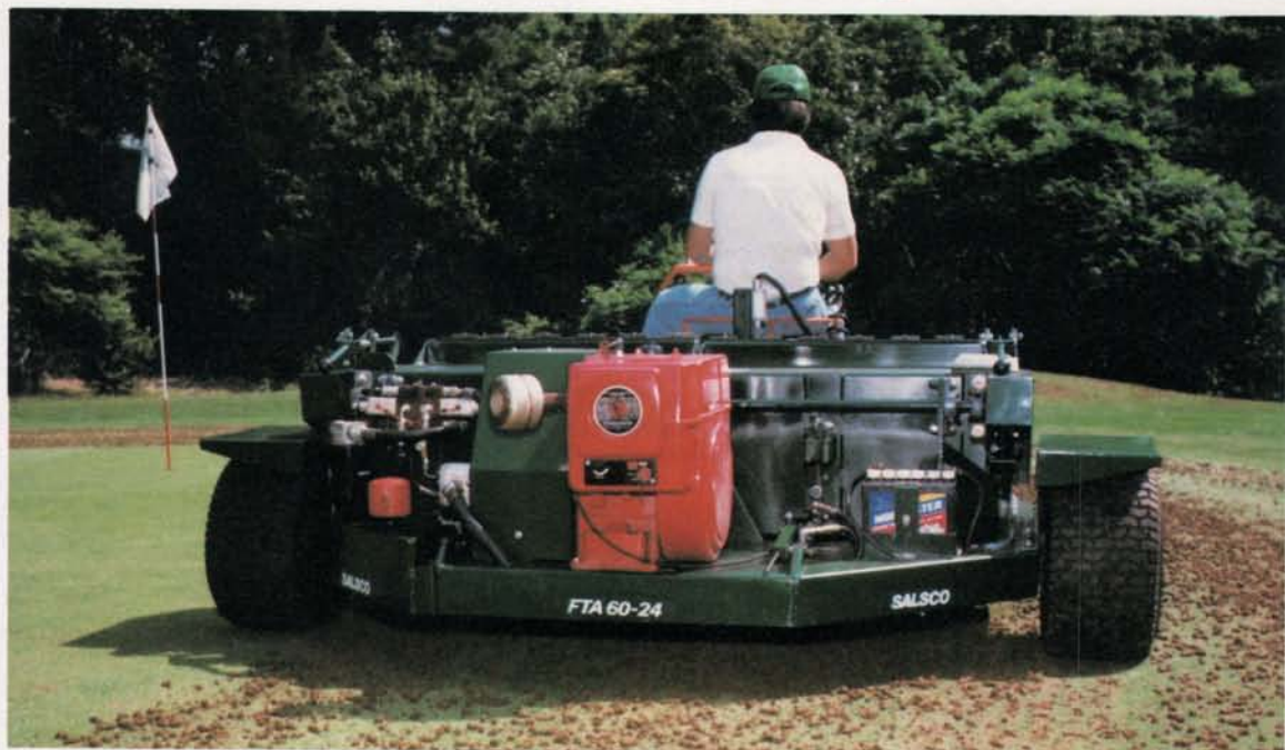
The FTA-60-24 Core Aerator can core up to 60,000 square feet per hour.
