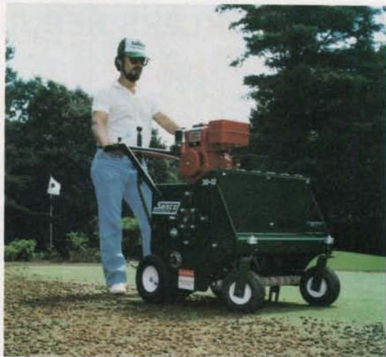
The 30-12 Core Aerator turns in a 15" radius while aerating.
