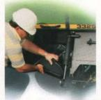
Frame design allows the 3325 to carry a fullsize grass catcher on the center cutting unit.
