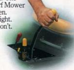
A single lever lifts all five cutting units simultaneously to make crosscutting easier.
