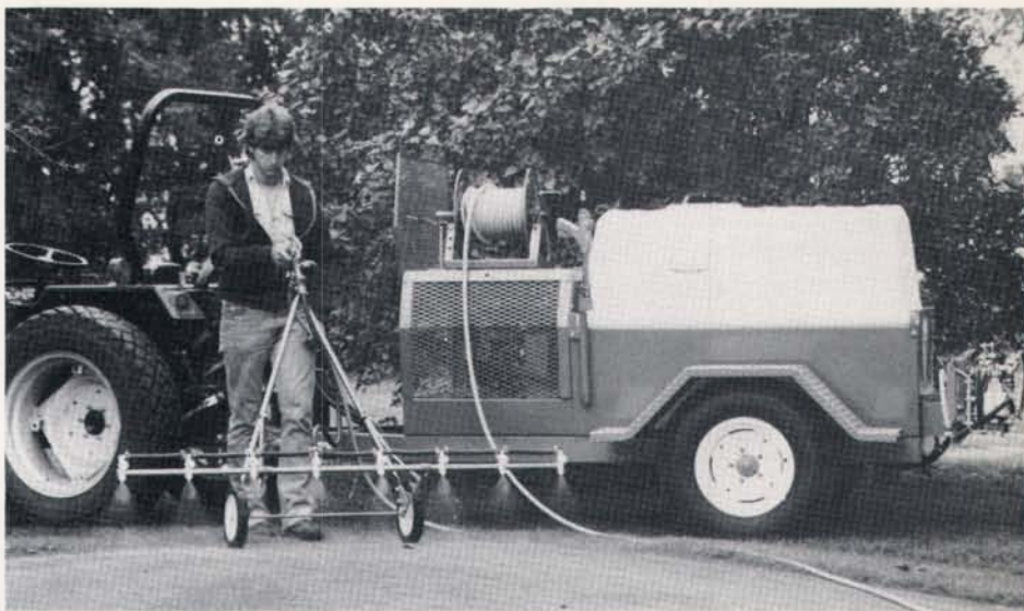
A walking boom sprayer and indicator dye can provide an extra level of certainty during pre-emergence herbicide applications.
