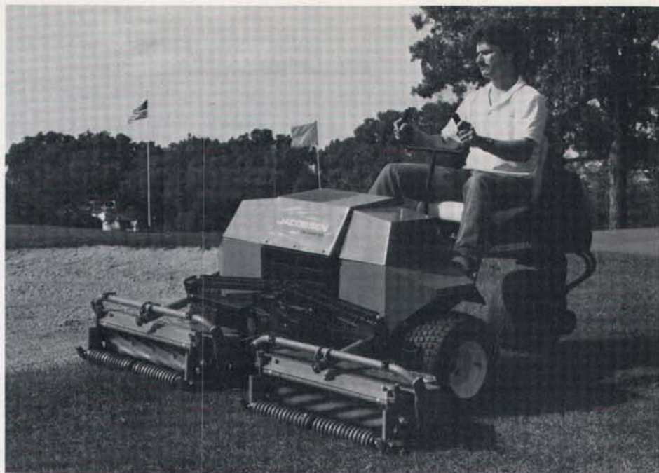
Three-wheel drive provides improved traction and maneuverability for Jacobsen's Tri-King 1471 triplex reel mower.
