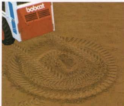
The Bobcat skid-steer loader can turn in its own tracks.
