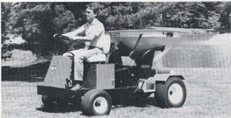
Large hopper pendulum spreader from Hahn is a fast way to topdress lightly.
