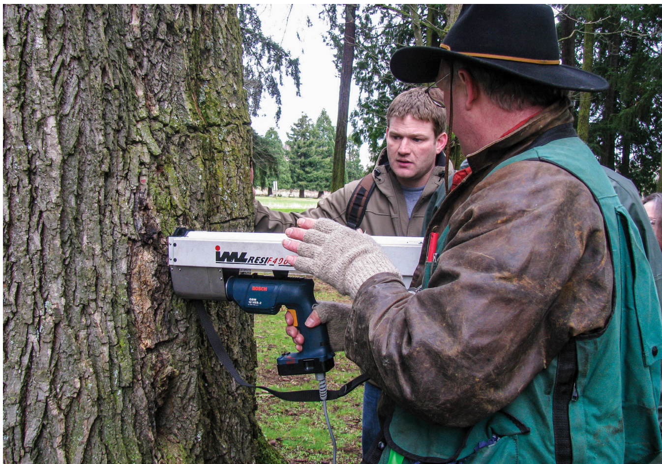
Use of a resistograph tool for advanced decay detection.
