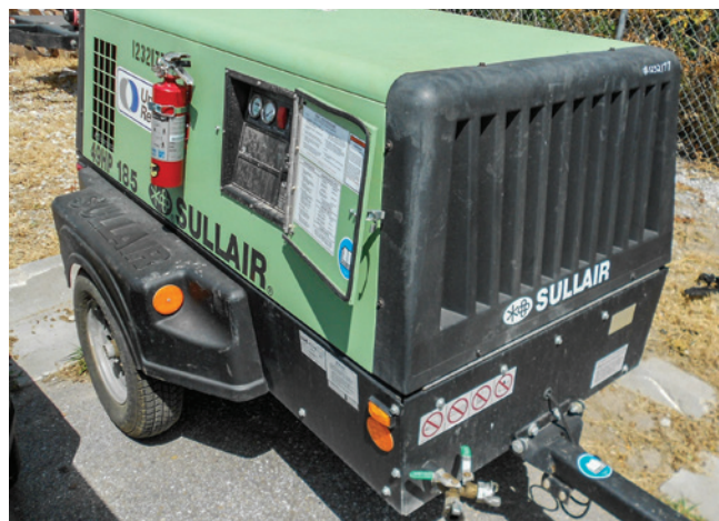
Figure 1: Example of a 49-hp air compressor with a 185-cfm capacity. The capacity is normally labeled on outer framework of the compressor.
