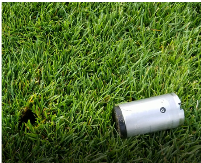
Figure 3. Catastrophic failure of sprinkler head due to too high air pressure and exit velocity.
