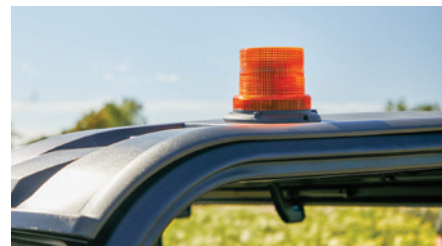
Lighting is an effective addition for increasing operator visibility and calling attention to the vehicle.
