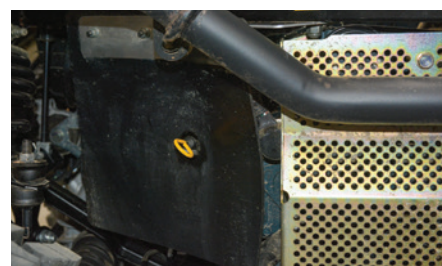
Mud guards help reduce exposure to mud, dirt and caustic chemicals in a UTV's driveline and engine bay.
