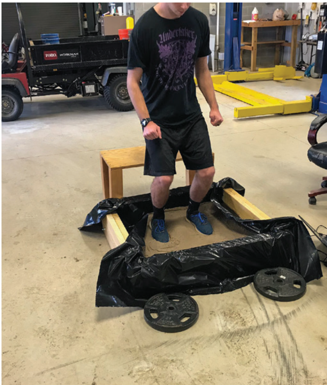
Figure 1. A novel ground reaction platform designed at the University of Georgia utilizes a mobile force plate to evaluate the interaction of athletes with various field playing surfaces.
