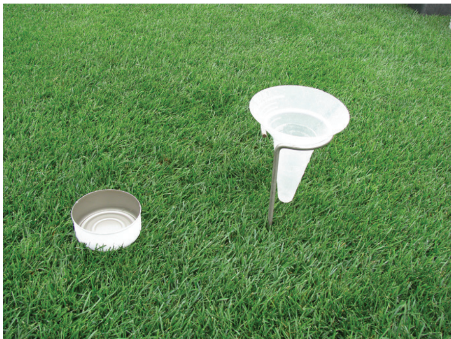
Collection cylinders and tuna cans work equally as well in the auditing process All photos by John C. Fech
