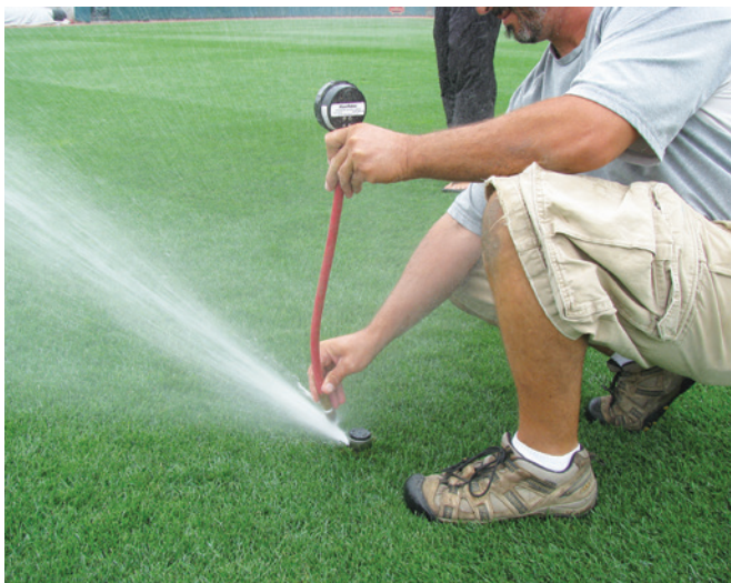
Checking water pressure with a pitot tube
