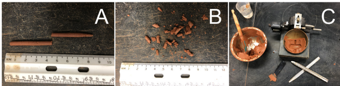
Figure 4: A. Soil above the plastic limit can be rolled into threads. B. The thread crumbles as it dries below the plastic limit. C. Soil paste flows at the liquid limit.
