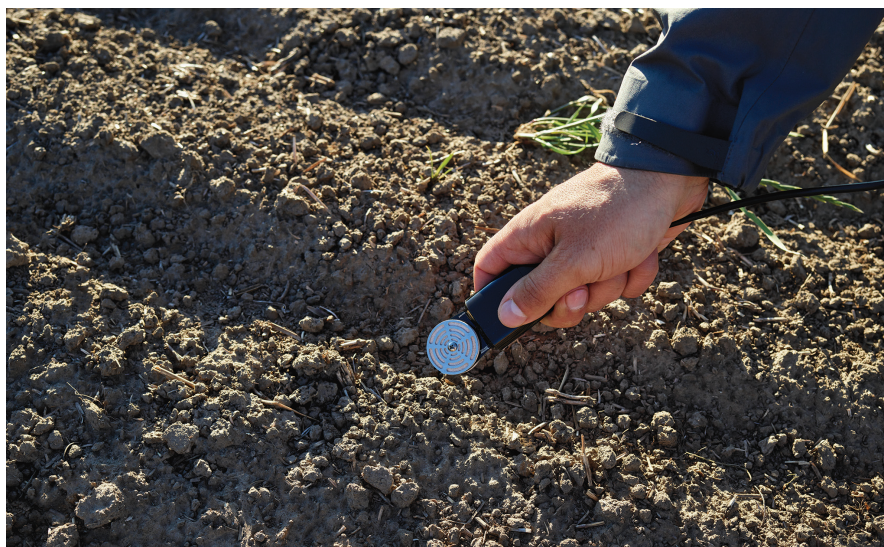
Figure 3: Soil water tension sensor, sometimes called a water potential or matric potential sensor
