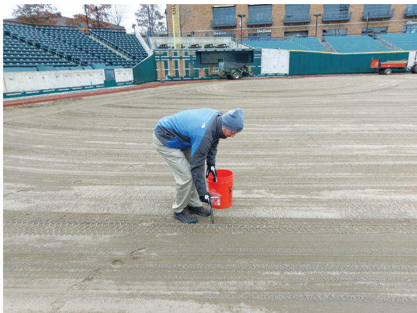
Soil tests professionally taken to analyze rootzone throughout the process.
