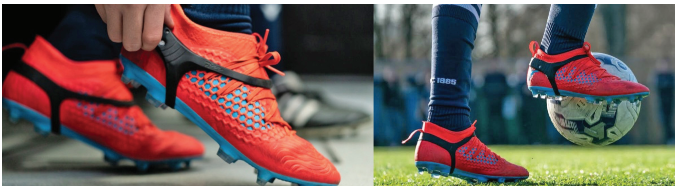
Figure 3. Example of an IMU fastened to back of soccer cleats with custom-made strap (PlayerMaker, Tel Aviv, Israel).
