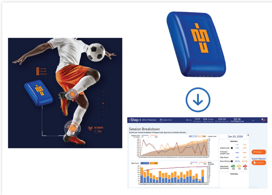
Figure 2. Example of an inertial measurement unit (IMU) placed on the lower leg (IMeasureU, Auckland, New Zealand). Data can be streamed in real time or downloaded after practices or games to a dashboard for further analysis. It is important to check the protocols for data security and Cloud storage of personal data, which may differ in each state or country.
