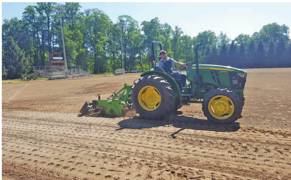
Tilling in soil amendments and punching holes for the sprigs to root faster. Photos provided by Kevin Mercer, CSFM, CGM, LICM
