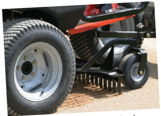
Center mounted is important. It's where most of the machine's weight is available to help dig into hard surfaces.
