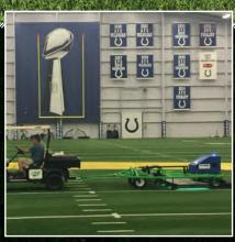
The GreenZapr tow-behind unit disinfecting the turf of a professional practice facility.
