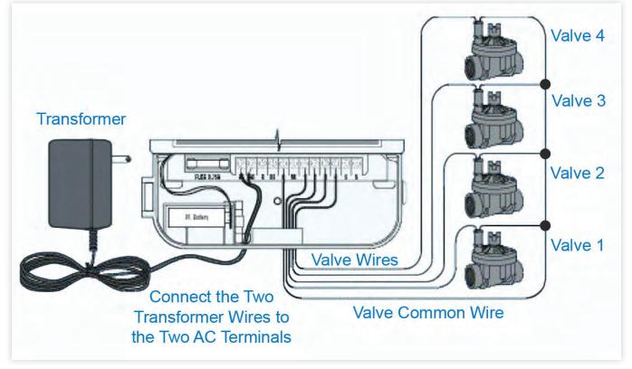
As you can see in the diagram above, each valve has two wires going into it. The common wire is connected to every valve, and is typically (but not always) a white wire. The other wire going into the valve is wired into one of the numbered terminals in the controller.
