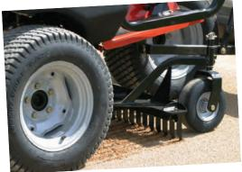
Center mounted is important. It's where most of the machine's weight is available to help dig into hard surfaces.
