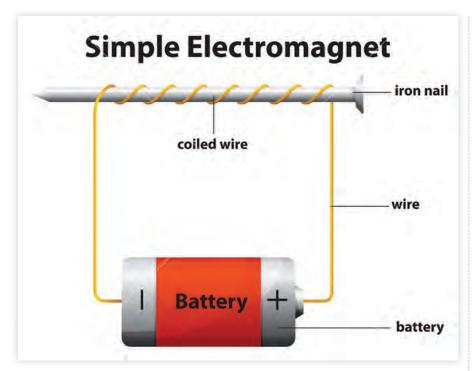
If you were to crack open the solenoid, you would notice that it is wrapped with extremely fine copper wire, similar to the electromagnet you might have made in 6th grade science class.
