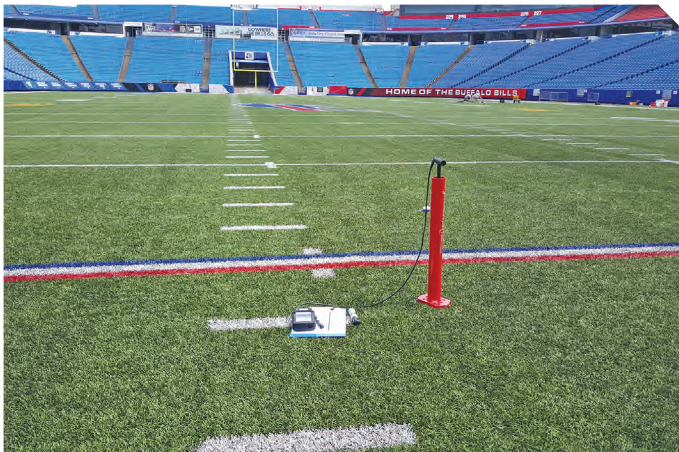
Monitoring surface hardness with a Clegg impact soil tester.
