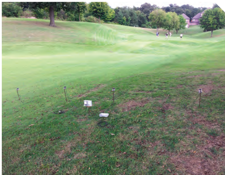
PAR sensors aligned to determine DLI quantities at positions where turf has full coverage, is slightly declining, significantly declining, and where turf has failed due to shade stress.
