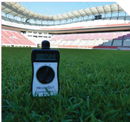
Spectrum FieldScout Quantum Light Meter being used in a stadium to measure PAR. Photo courtesy of Micah Woods, PhD.
