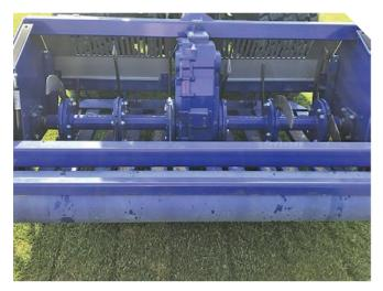
Figure 6. The Imants ShockWave can be used to incorporate some topdressing sand into the rootzone while causing minimal amount of disruption to the playing surface.
