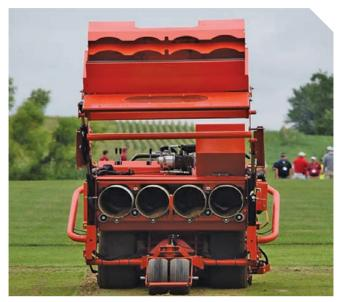
Figure 5. The Wiedenmann Core Recycler separating the organic matter and sand from hollow tine cores on athletic field turf.
