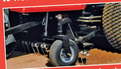
Spring tine scarifier chews into surfaces but skims over base spikes or pockets.
