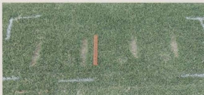
The Pennswing divot resistance tester (left); examples of small divots (above) and large divots (below) produced by Pennswing, with 12-inch ruler for scale.
