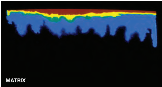
▲ Thermal imaging shows water moving in a fingered flow through water repellent soil (top) and the desired matrix flow in a non-repellent soil (bottom).
