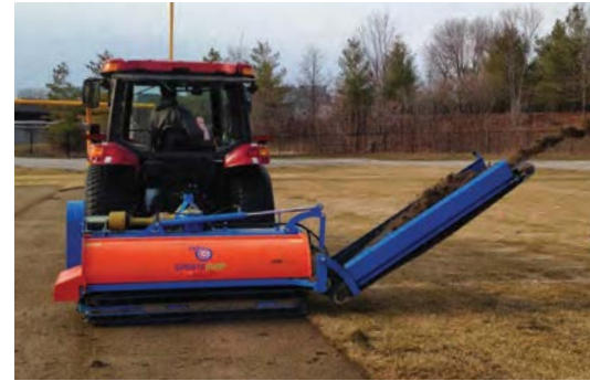
Fig. 6. Fraze mower used to remove grass and the upper layer of soil from practice sports field at Iowa State.
