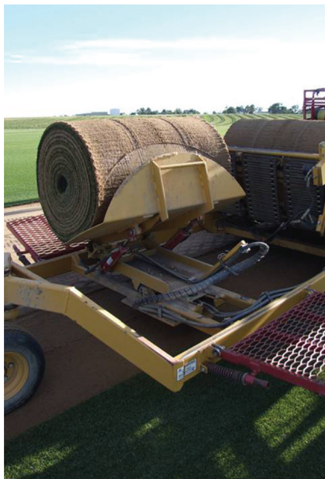
▲ The back of the 4-foot harvester with two harvested rolls on the back of the machine.
