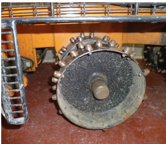
▲ Cleats on wear machine at the Sports Turf Research Institute, Bingley, England
