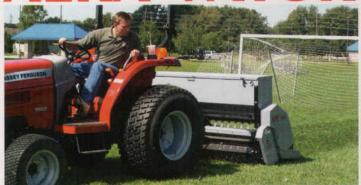
One machine, One pass. Aerate and overseed at the same time. With an optional slicer shaft and multi-tine shaft,
