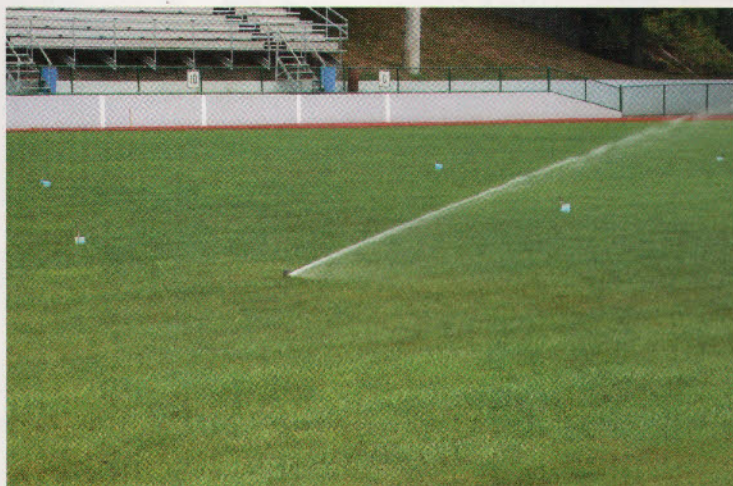
The catch-can devices that you use for capturing precipitation should be uniform and level.
