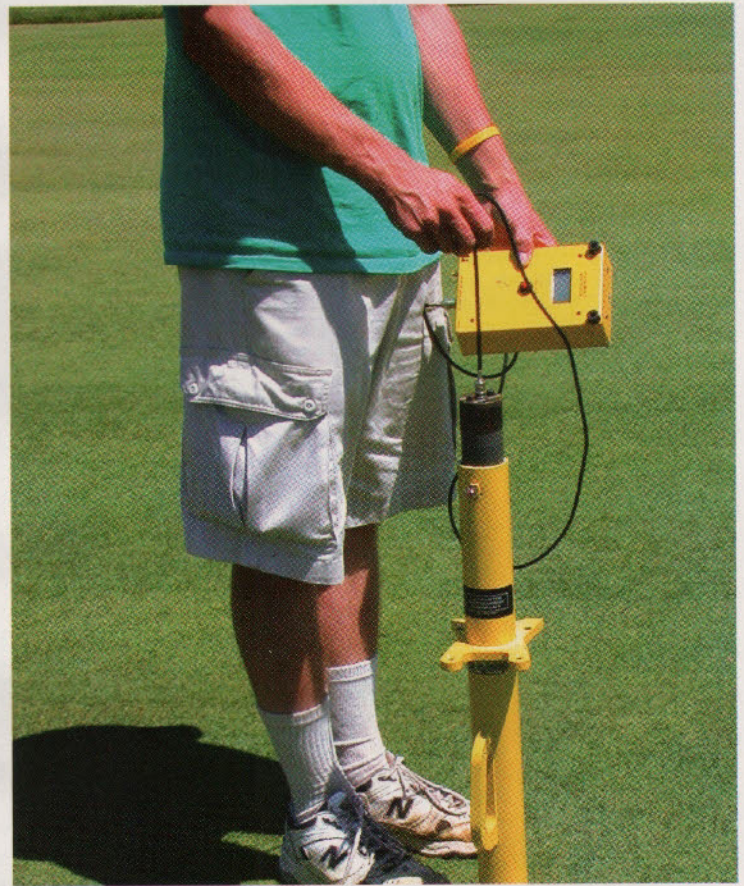
Figure 1A and 1B. Impact tester used for synthetic turf testing (A) and for natural turf and soil testing (B).
