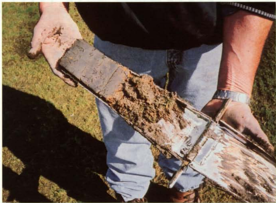
It was important that the topsoil (growing medium) was thoroughly blended with the subgrade to prevent layering.
