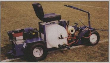
The Jaydee Drive Liner is a self-propelled riding line marker. The 35-gallon paint tank carries enough marking material for a complete game field, or several practice fields. The 2-gallon flush tank cleans the discharge lines for work breaks, travel, or overnight. The center or side-mark spray shields are always operator-visible. A nearly zero turning radius reduces or eliminates back and turn maneuvers.
