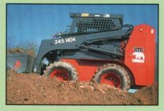
and built to withstand the stress of high-impact shock loading, day after day. A wheelbase of 44.8 inches provides smooth, stable operating regardless of terrain. An optional high-flow hydraulic package is also available to power attachments such as large cold planers, rock saws and trenchers.
