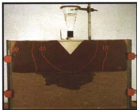
In a fine soil overlying a coarser, free-draining layer, water is held in, resulting in a perched water table. Courtesy: Lanco
