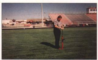
The Clegg Impact Soil Tester is the "instrument of choice" for both natural and artificial turf (ASTM #F1702-96). The Clegg is used to measure the "stiffness" of natural or constructed conditions. Control the safety and playability of your field with our reliable and accurate device. For a representative in your area please call:
