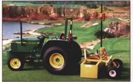
For level, single, or dual grade, GRADEMASTER is automatically laser controlled and eliminates uneven grade, potholes, wet spots and dips on athletic fields, greens or tee boxes. GRADE-MASTER . . . The Right Choice for your Grading applications. GRADEMASTER is easy to use! One man can operate GRADEMASTER and achieve improved accuracy. For information and video contact:
