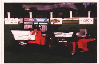
A new line for all 3-wheel groomers and all utility sports field vehicles. Easy Mount® slip in-slip out bracket. Plexiglass blow back shield. Remote electric toggle switch for open and close efficiency. 90° side plate for controlled coverage. All-weather plastic cover. Also fits Easy Mount® spray tanks, base holders, and hose reels. Fits Toro Infield Pro 5000, John Deere Bunker Rake 1200A, Smithco Super Rake, Chetech and others. Call for free catalog of other unique attachments and tools.
